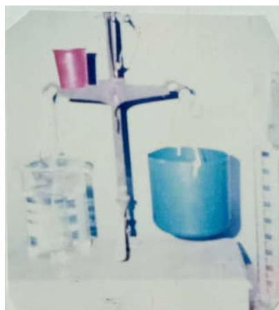
Figure 1 Instrument used in Wilhelmy Plate Method
