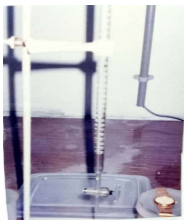
Figure 3 Instrument used in Falling Ball Method
