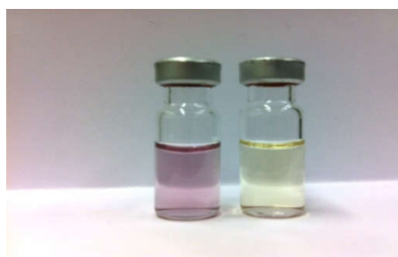
Fig 3 Reaction of compound with DPPH (violet) to 1,1'-diphenyl-2-(2,4,6-trinitrophenyl)hydrazine (yellow).
