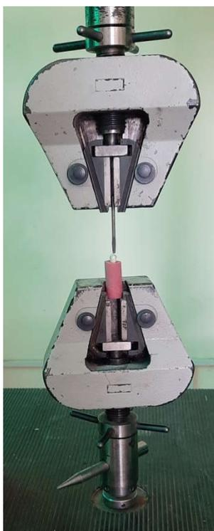
**Figure 3** Load applied on the teeth in Universal Testing Machine
