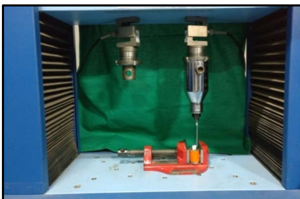
Figure 1 Sample Subjected to Load for Measuring the Tensile Bond Strength
