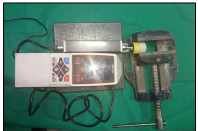
Figure 2 Sample Being Tested for Surface Roughness with Profilometer
