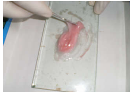
Figure 10 mixing of soft lining material
