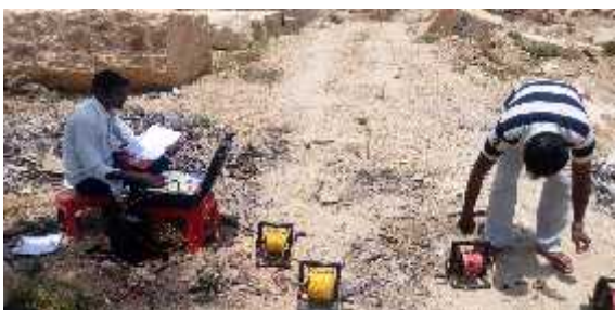
Fig 1 Resistivity Field survey in Arasiramani granite quarry
