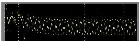
Fig. 29 Power Factor for Input = 100 V PF = 0.3
