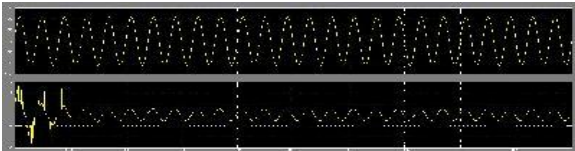
Fig. 14 Input Voltage & Current for Input = 100 V PF = 1
