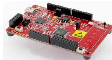
Figure 6 PSoC4 development board
