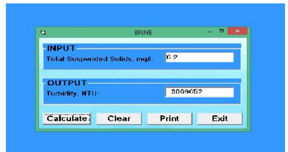
Figure 5 Software Determination of NTU of Brine at given TSS
